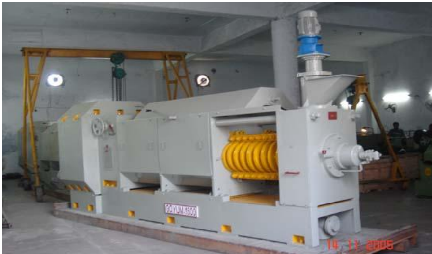
Figure 4: Goyum 1500 Long Cage 50 Ton/day Expeller with three cage sections
