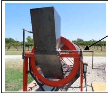
Figure 2. Hand crank pomace breaker/feeding mechanism. Motor placement at the crank brace is requested to correct uneven cleaning screen pomace delivery and decrease operator fatigue.
